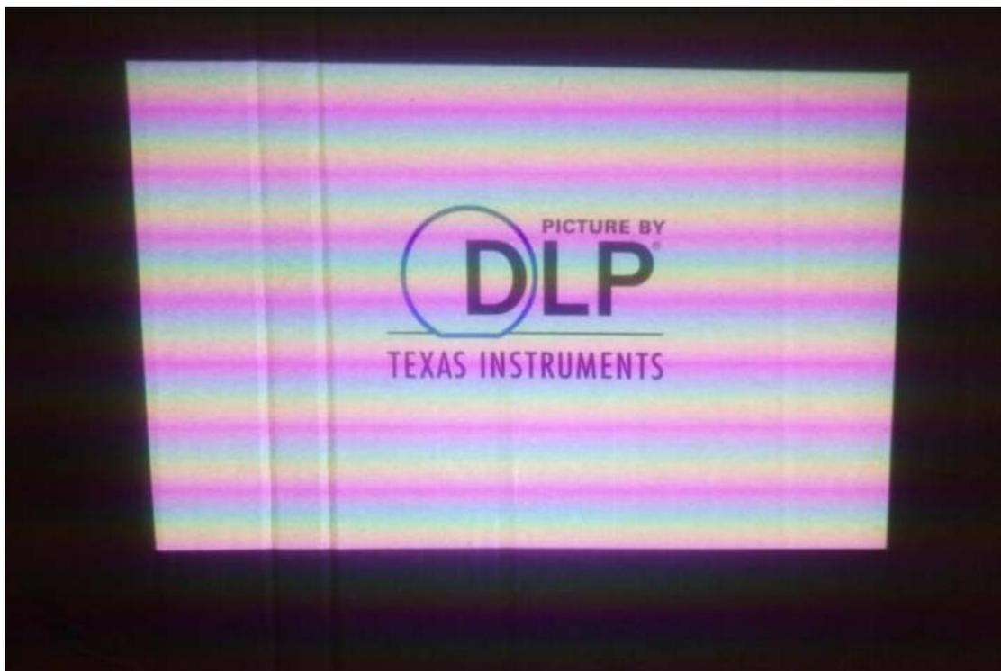
After the upgrade is complete (has been parked in the boot logo), press two times on the remote control shutdown button, and then wait until the machine shut down, pull out the U disk, turn off the power. And then turn on the power, press one time on the remote control boot button, wait until the machine boot on.
