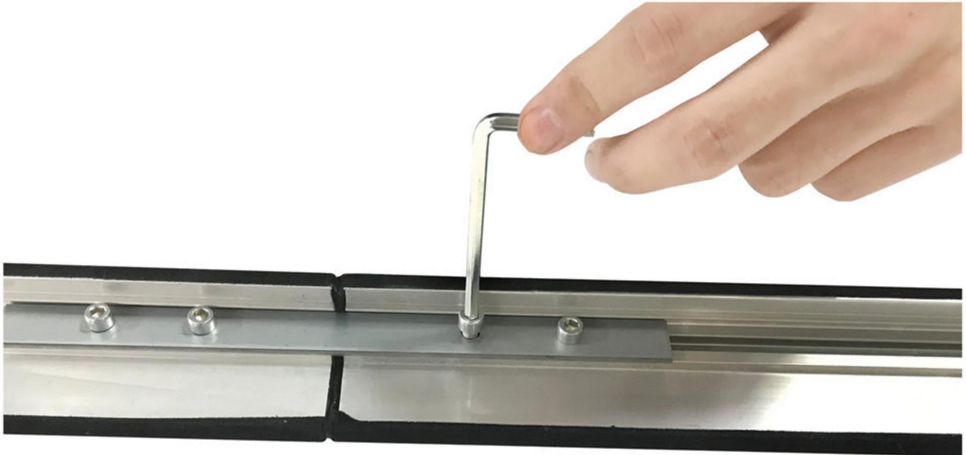
4> Take out another 2 pieces NO.3 frame, and please repeat step 1> to step 3> to make 2 pieces NO.3 frame together; After finish step 4>, you will get 2 long pieces frame which length is 231cm,,we can call this frame which is 231cm name is NO.21 Frame
